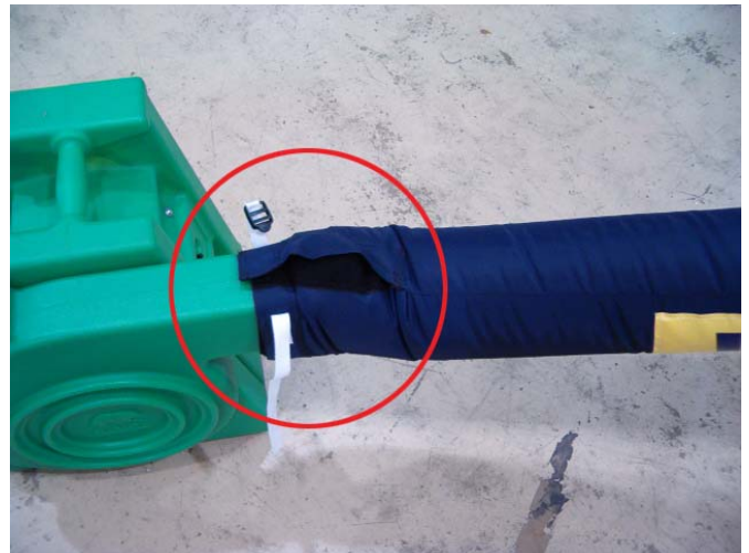
The inflation tube attaches to the blower as shown. Be sure to tighten the nylon strap to secure the inflation tube before activating the blower
