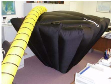
It measures 6' x 6' x 5' high and is supplied with 25' of 8" diameter flex duct and one 120V-2 HP blower. The blower must remain on at all times to keep the platform inflated.
