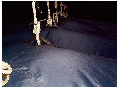
2. Balloon hangs from a rod that extends from one point on the stack to another 180 deg away. Think of a curtain rod
